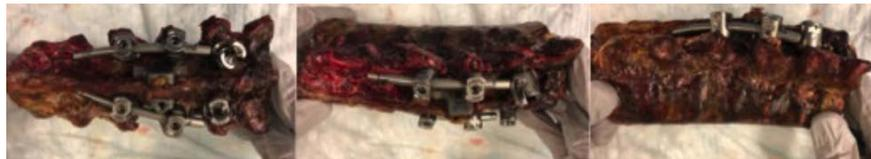
**Figure 2.** Construct 2 with pedicle screw instrumentation and rod fixation at T8 and T9 with an IFC between T7 and T8.
